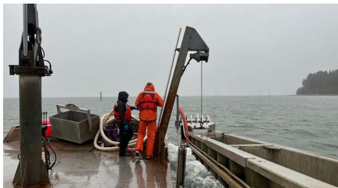
Figure 2. Prototype precision harvest arm mounted on the boat.
